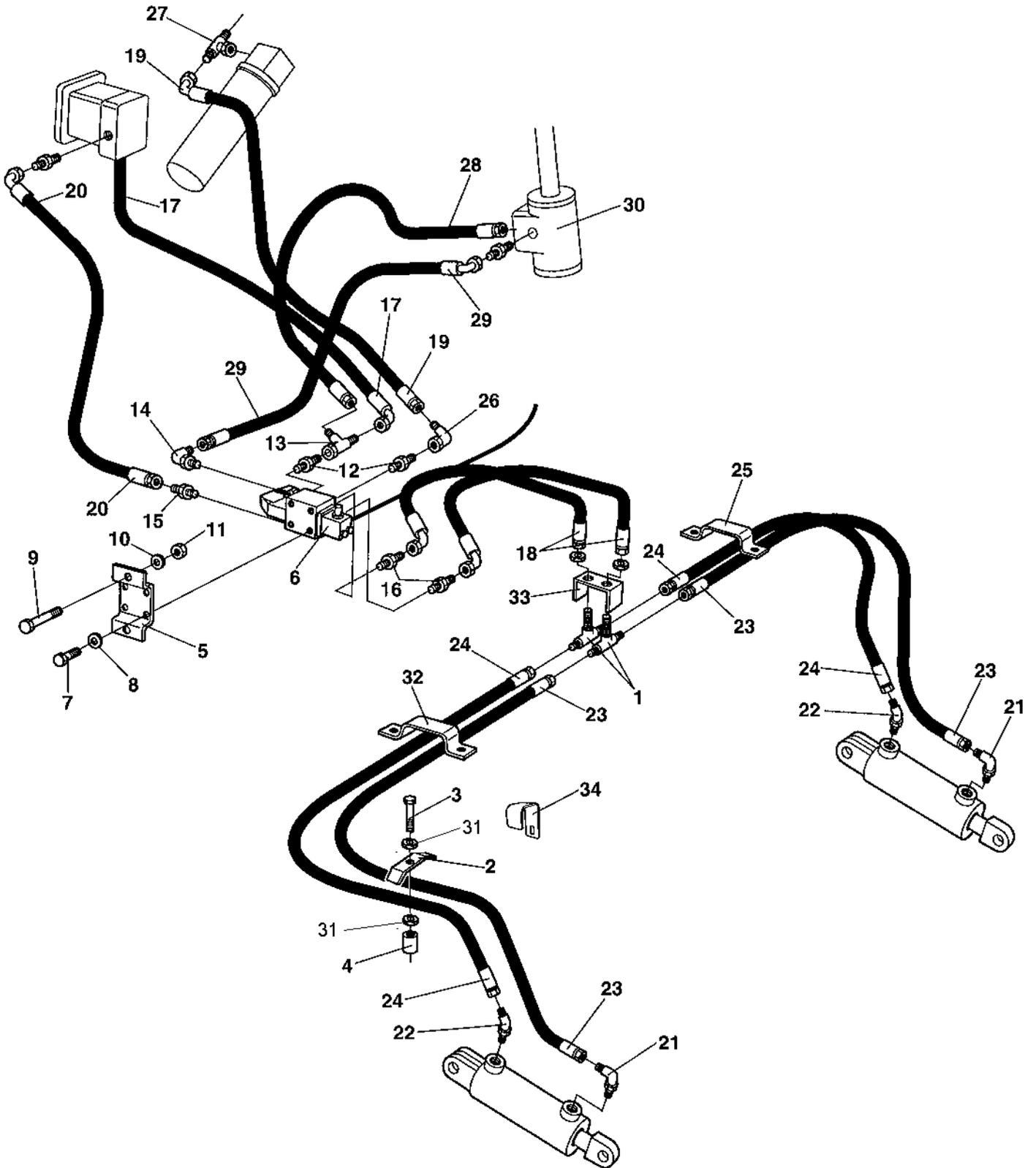
Levelling blade, hydraulic parts
