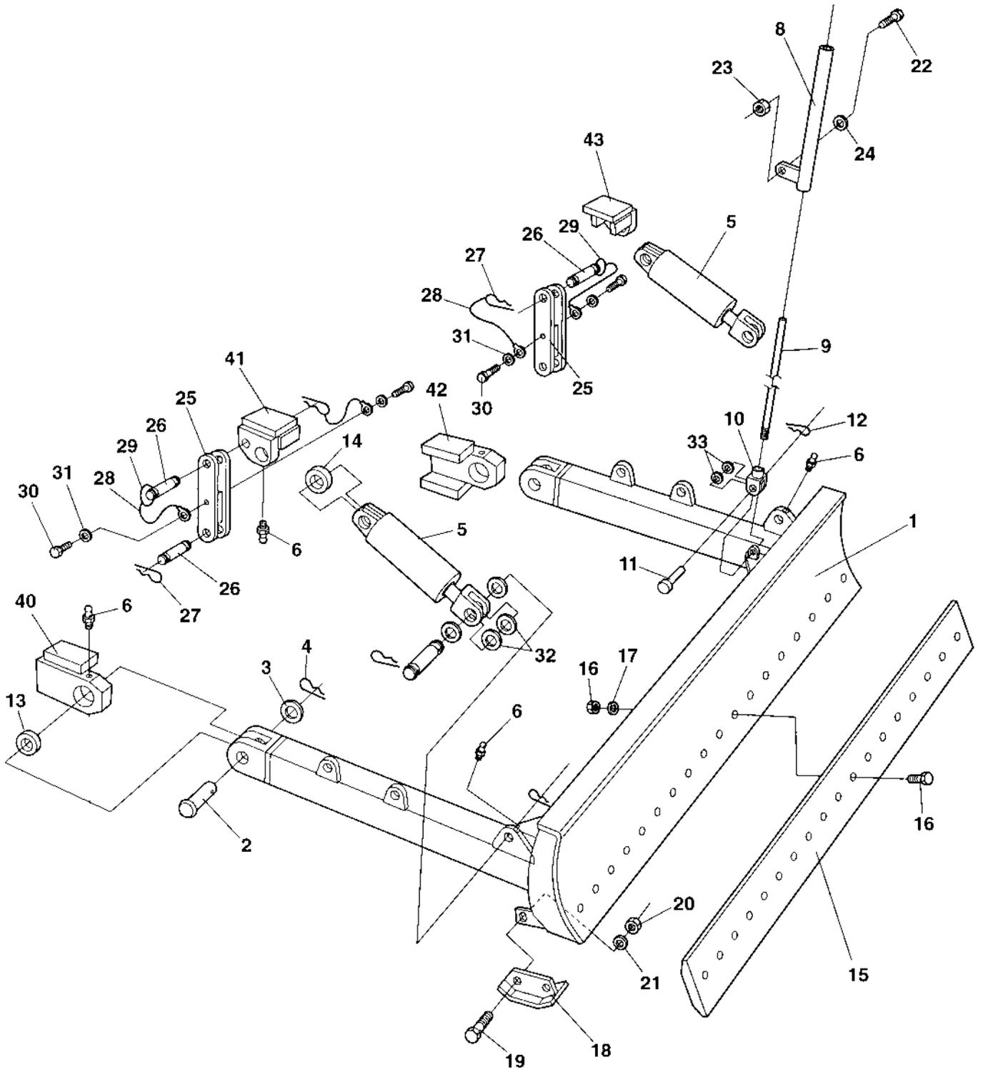
Levelling blade, metal parts
