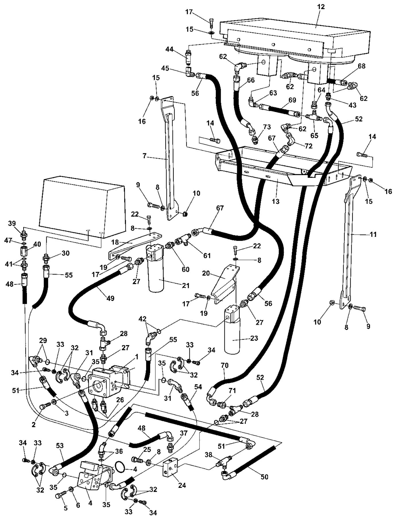
**Propulsion and Oil cooling system, Rear**
