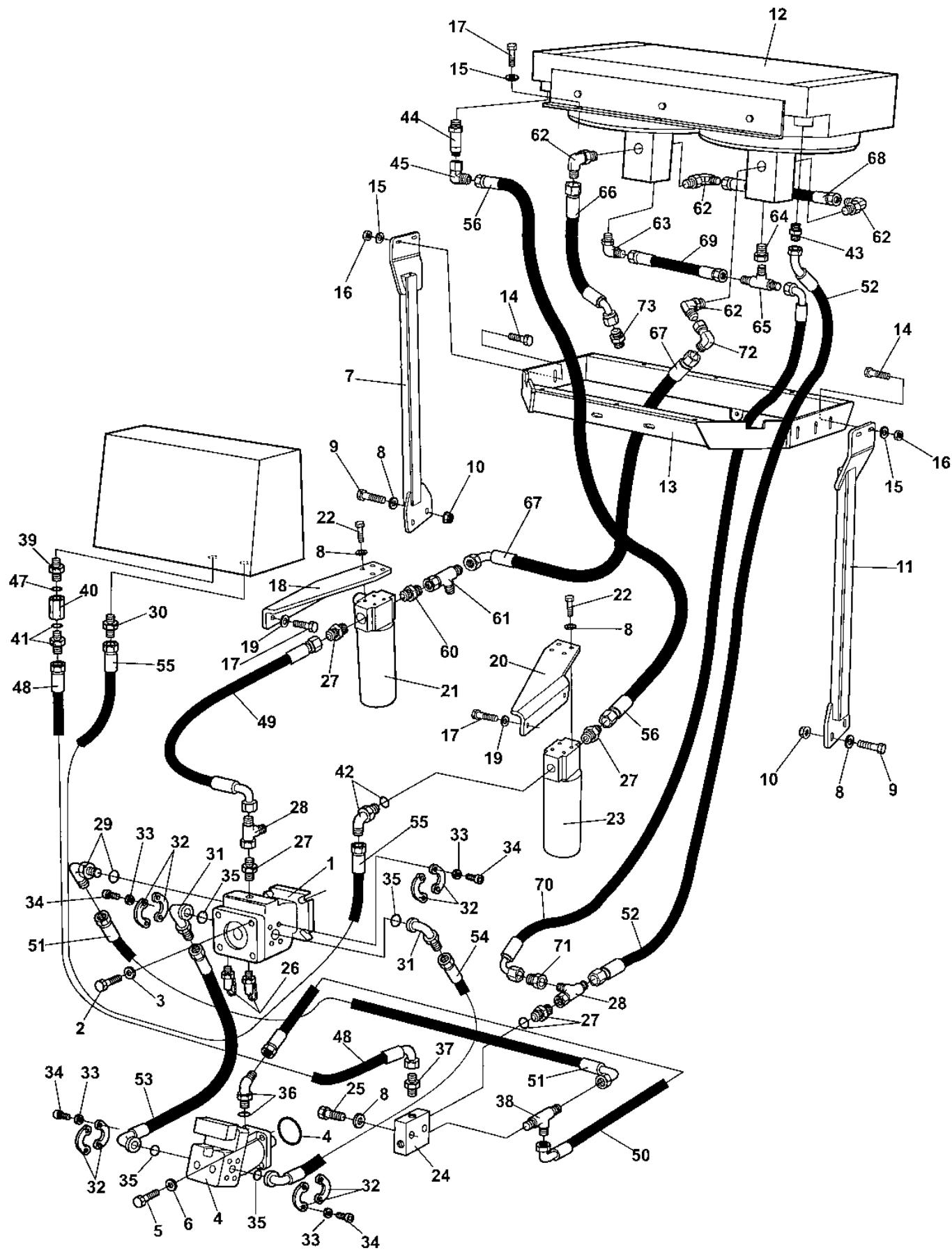
**Propulsion and Oil cooling system, Rear**
