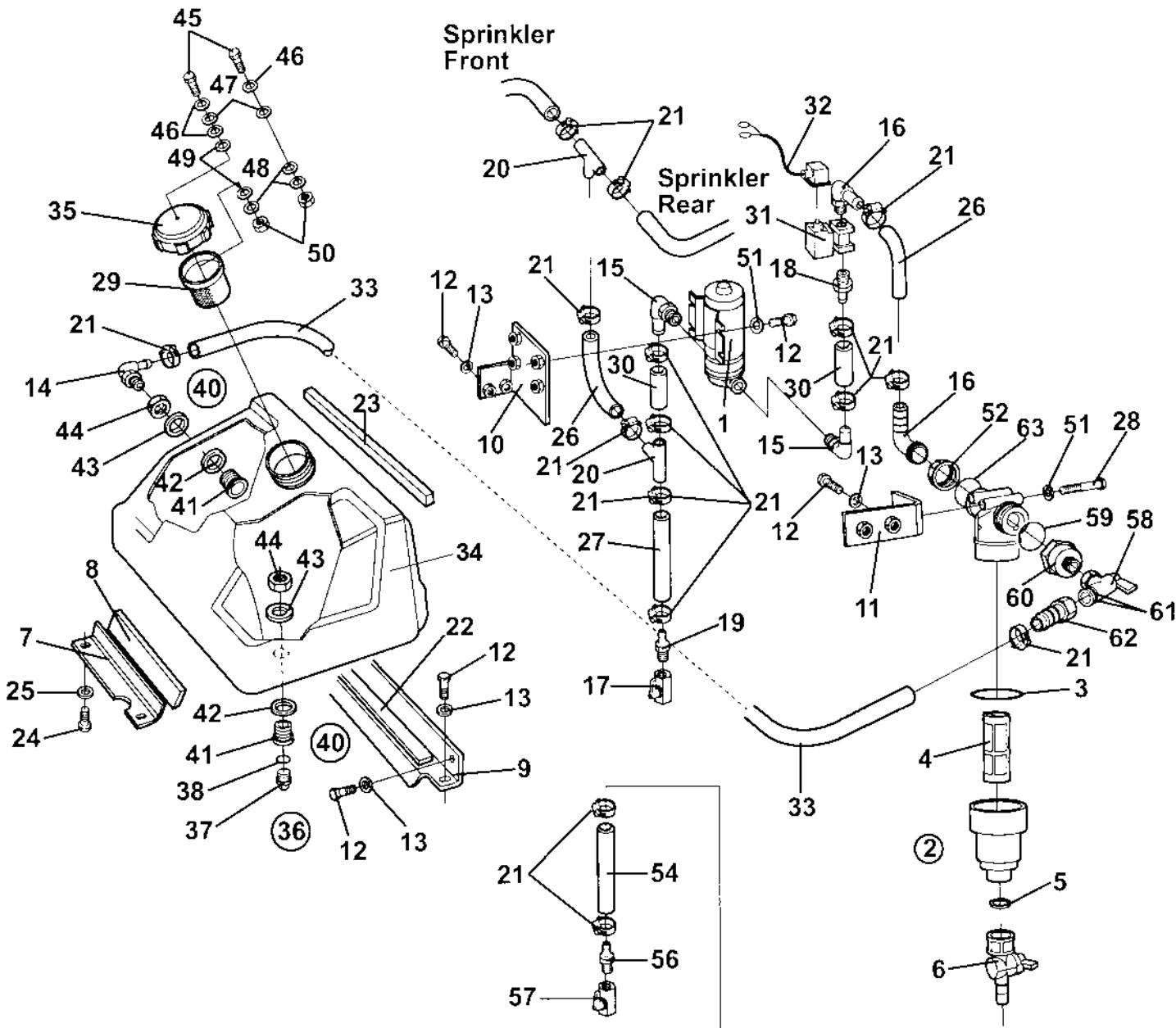
**Sprinkler system Front tank**
