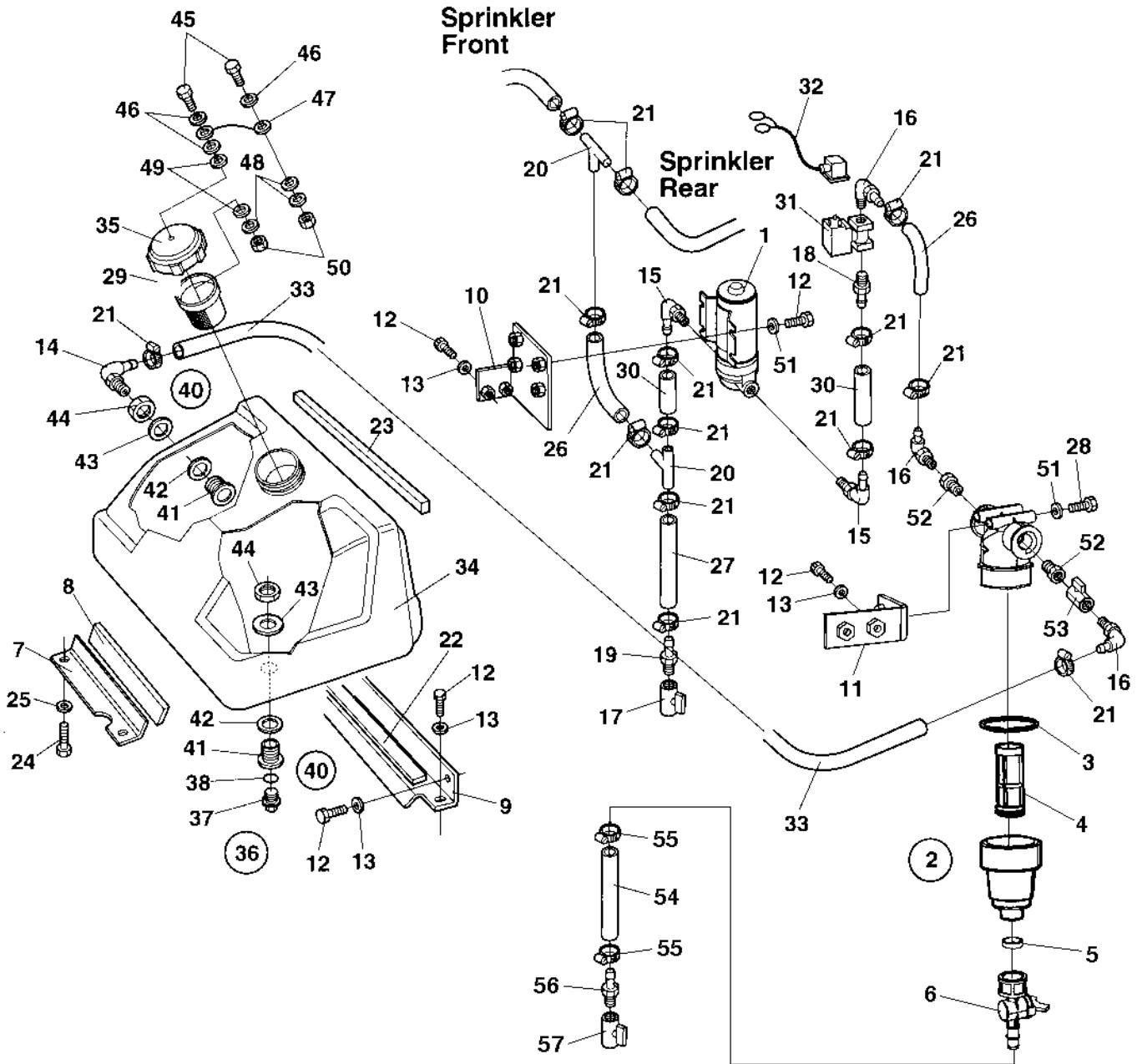
Sprinkler system Front tank
