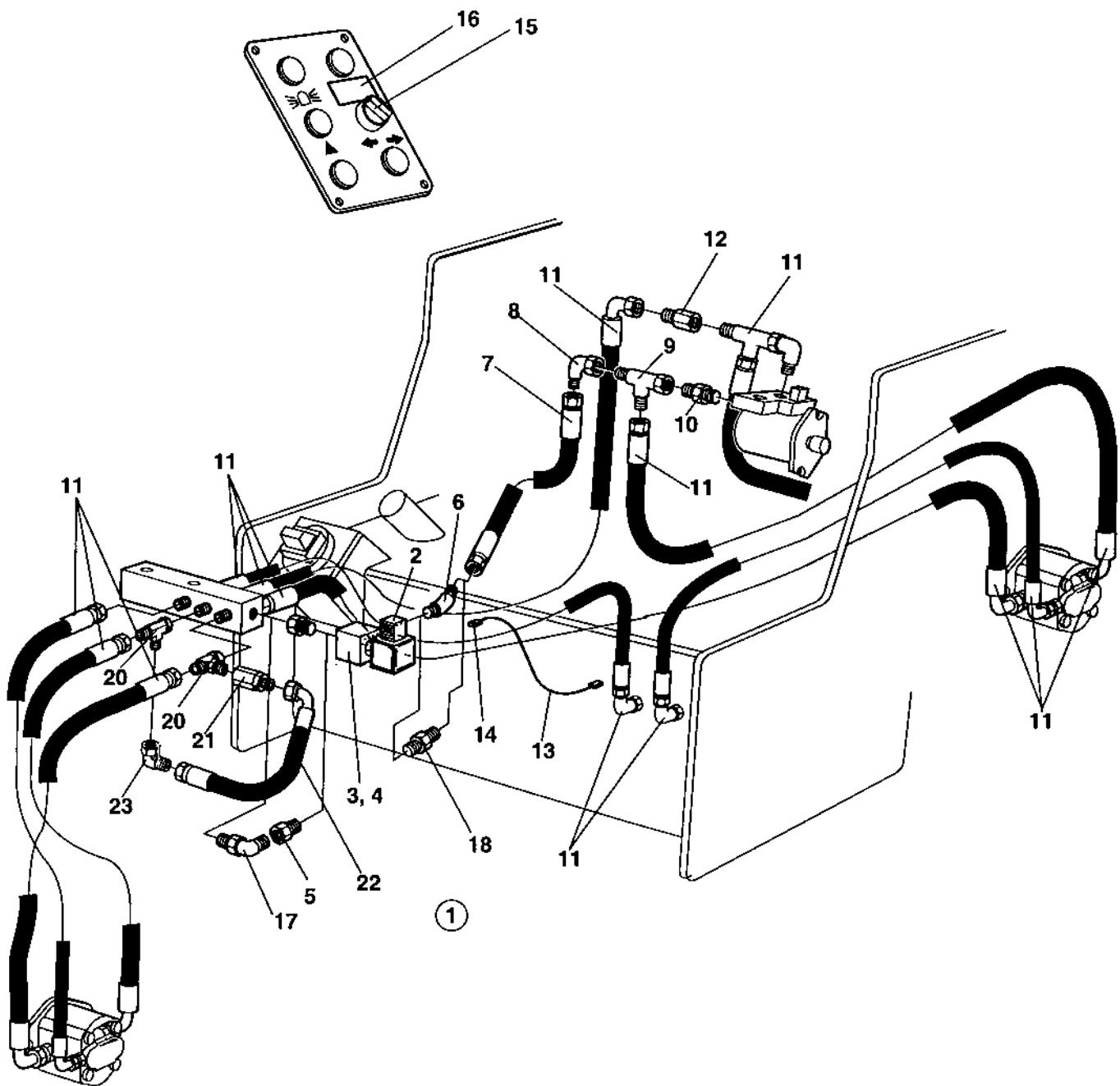
Vibration shut-off, front drum DEUTZ
