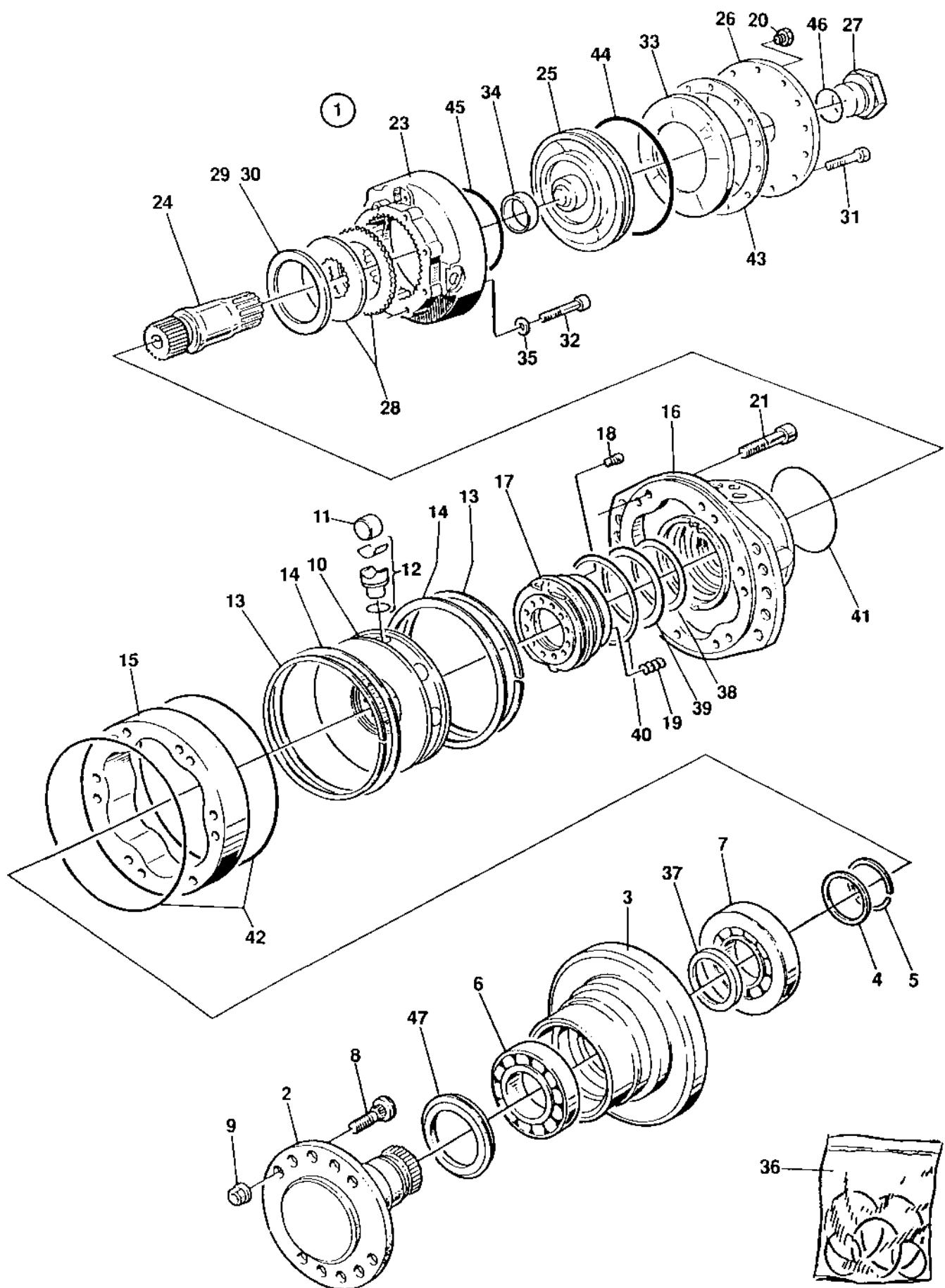
**4700375631 Hydraulic motor, propulsion, drum**
