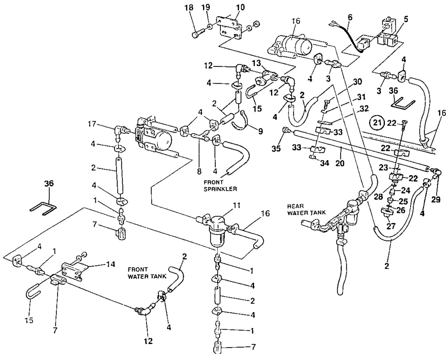
Combination water supply 2 rear sprinkler pipes
