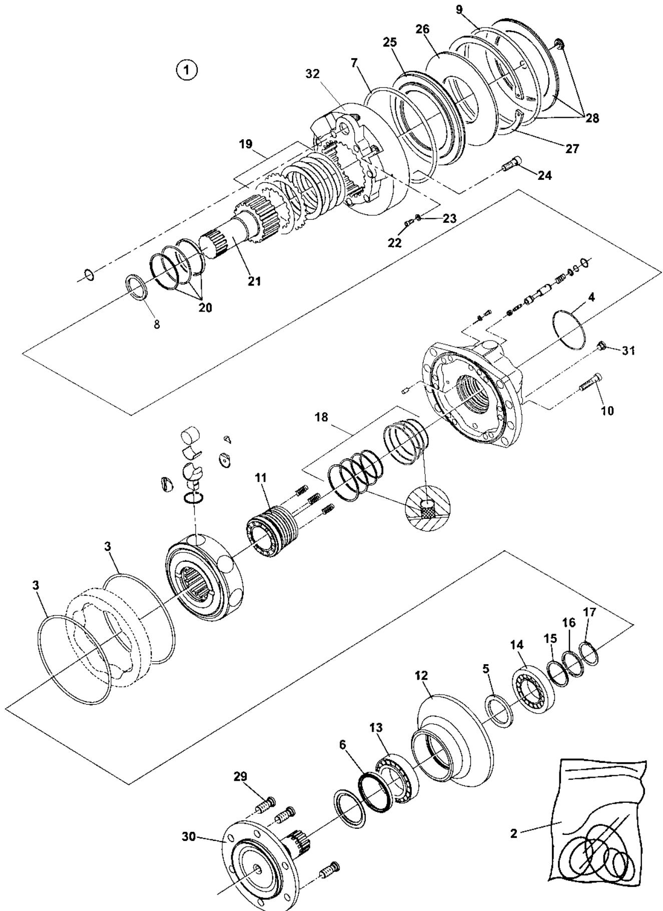
**4700390742 Hydraulic motor, propulsion, drum**
