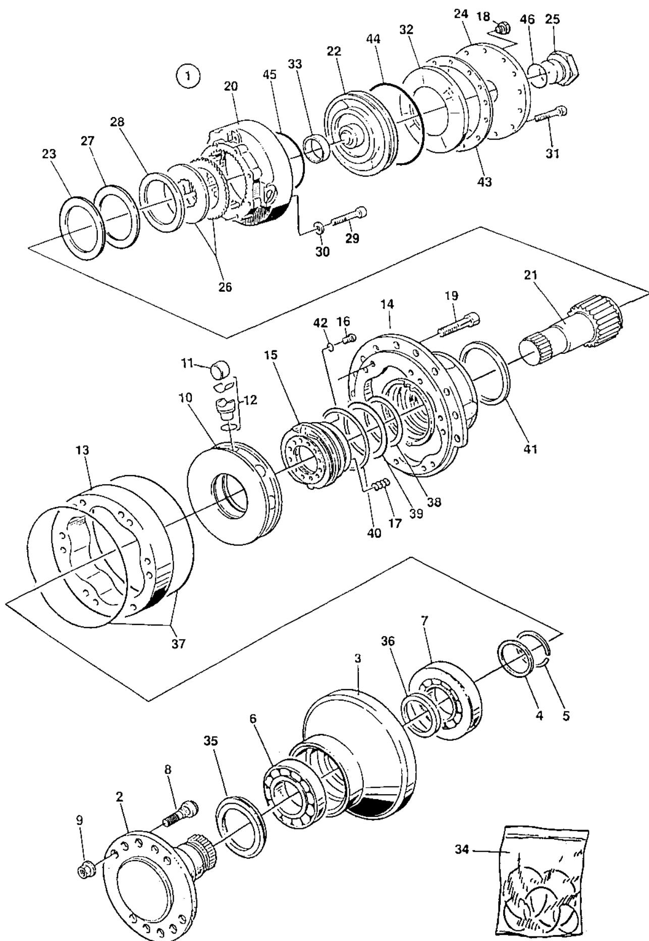
**4700372118 Hydraulic motor high torque**
